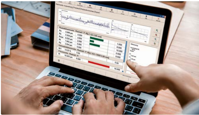
“Evaluation” screen: Result with profile, AD curve, Mr curve and tolerance monitoring
