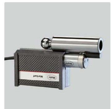
Measurements of end faces of workpieces
