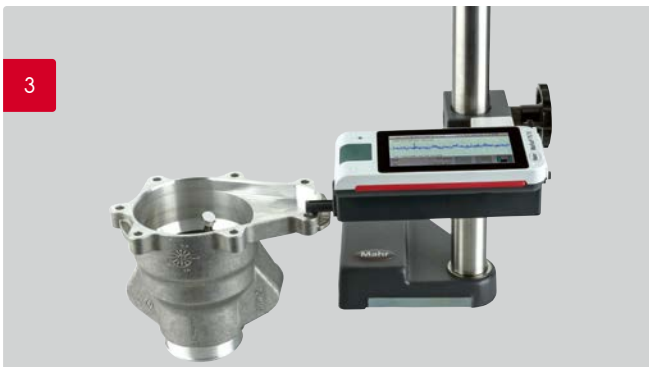
3. Roughness measurement with measuring stand ST-D
